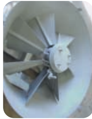
Internal drive Variable Inlet Vane (VIV). Cost effective design.
