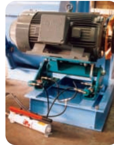
Hydraulically adjustable belt tensioning device
