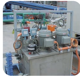
Automatic lubrication system designed to meet American Petroleum Institute (API) standards.
